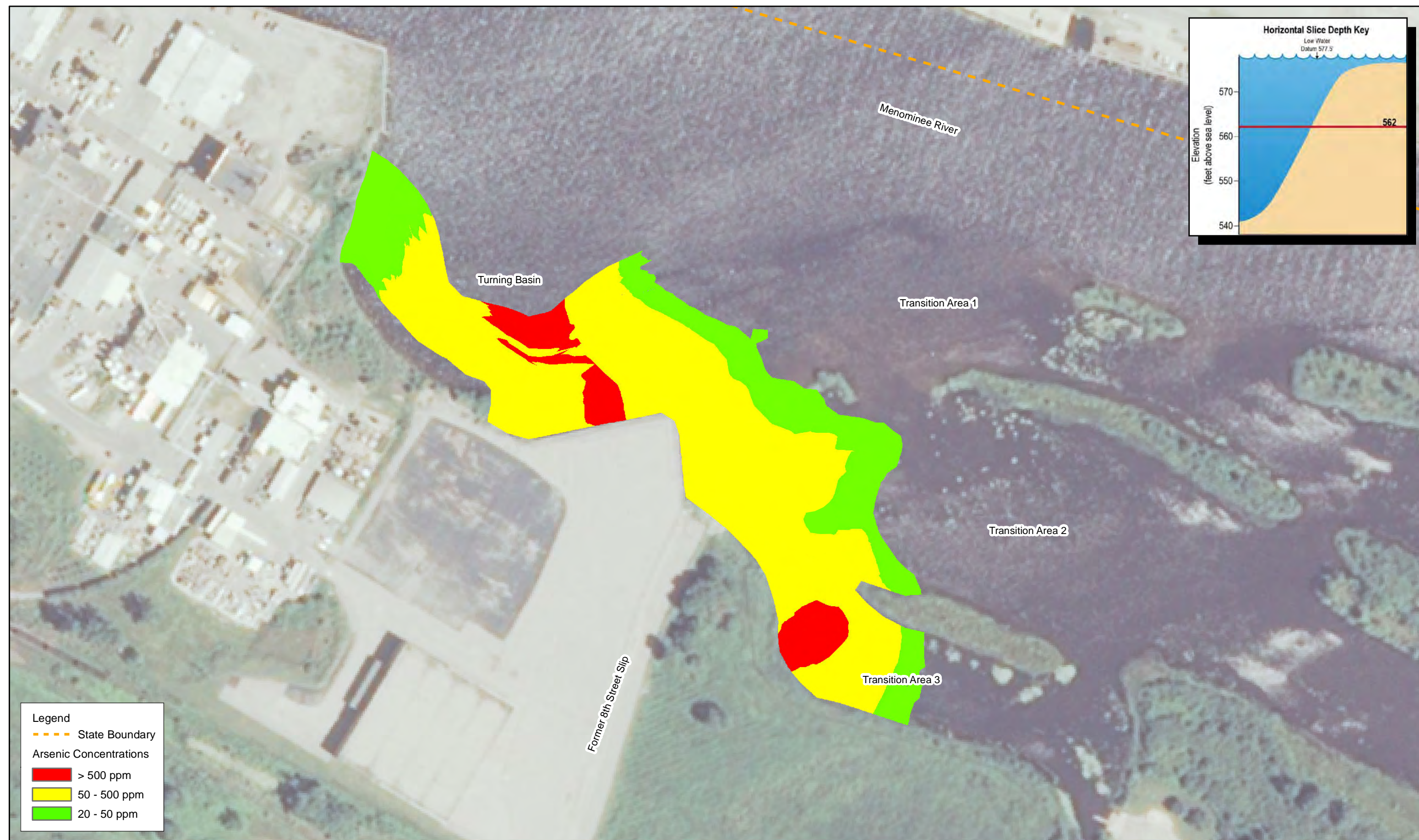
Figure 151 Horizontal Slice of Project Area, Arsenic Concentrations Elevation 562' Tyco Fire Products LP Facility Marinette, WI
