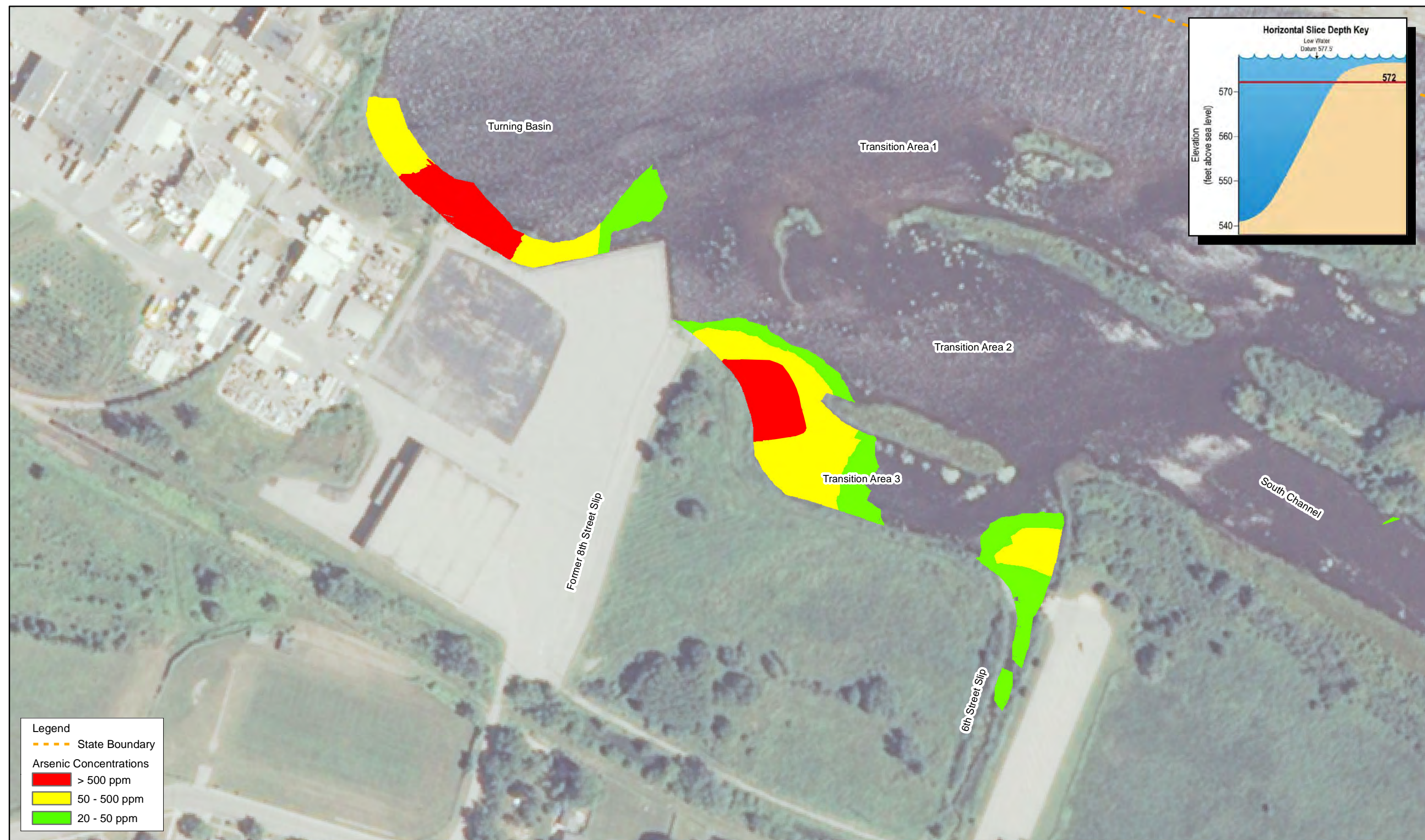
Figure 15N Horizontal Slice of Project Area, Arsenic Concentrations Elevation 572' Tyco Fire Products LP Facility Marinette, WI
