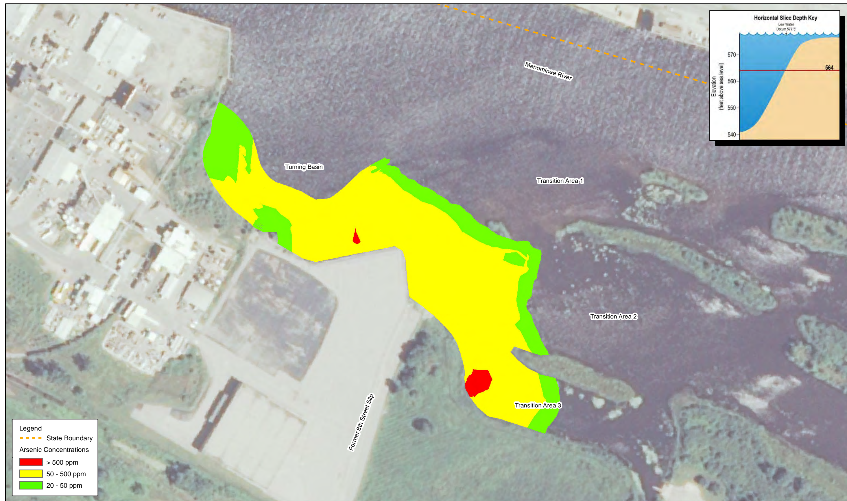
Figure 15J Horizontal Slice of Project Area, Arsenic Concentrations Elevation 564' Tyco Fire Products LP Facility Marinette, WI
