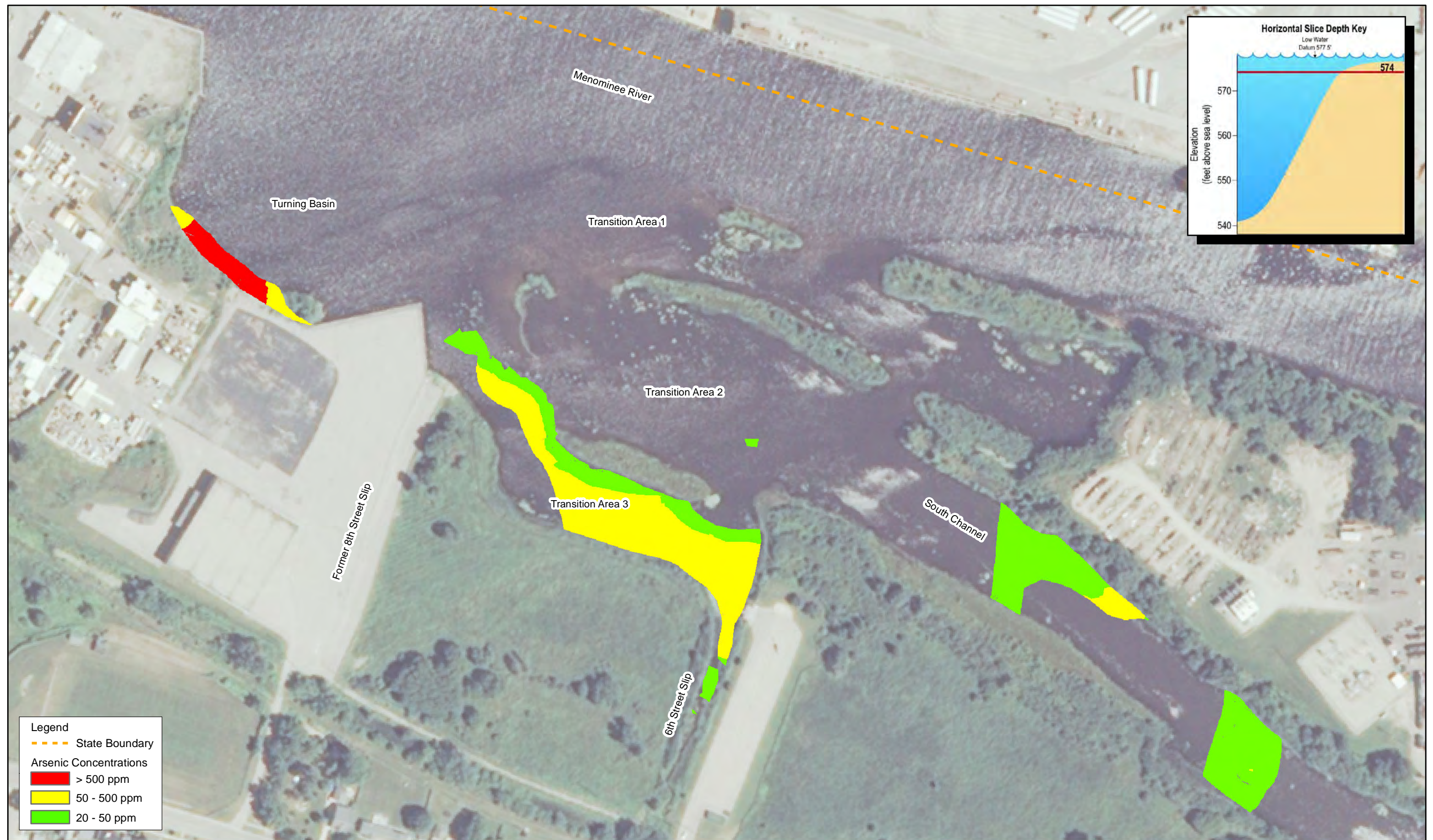
Figure 150 Horizontal Slice of Project Area, Arsenic Concentrations Elevation 574' Tyco Fire Products LP Facility Marinette, WI
