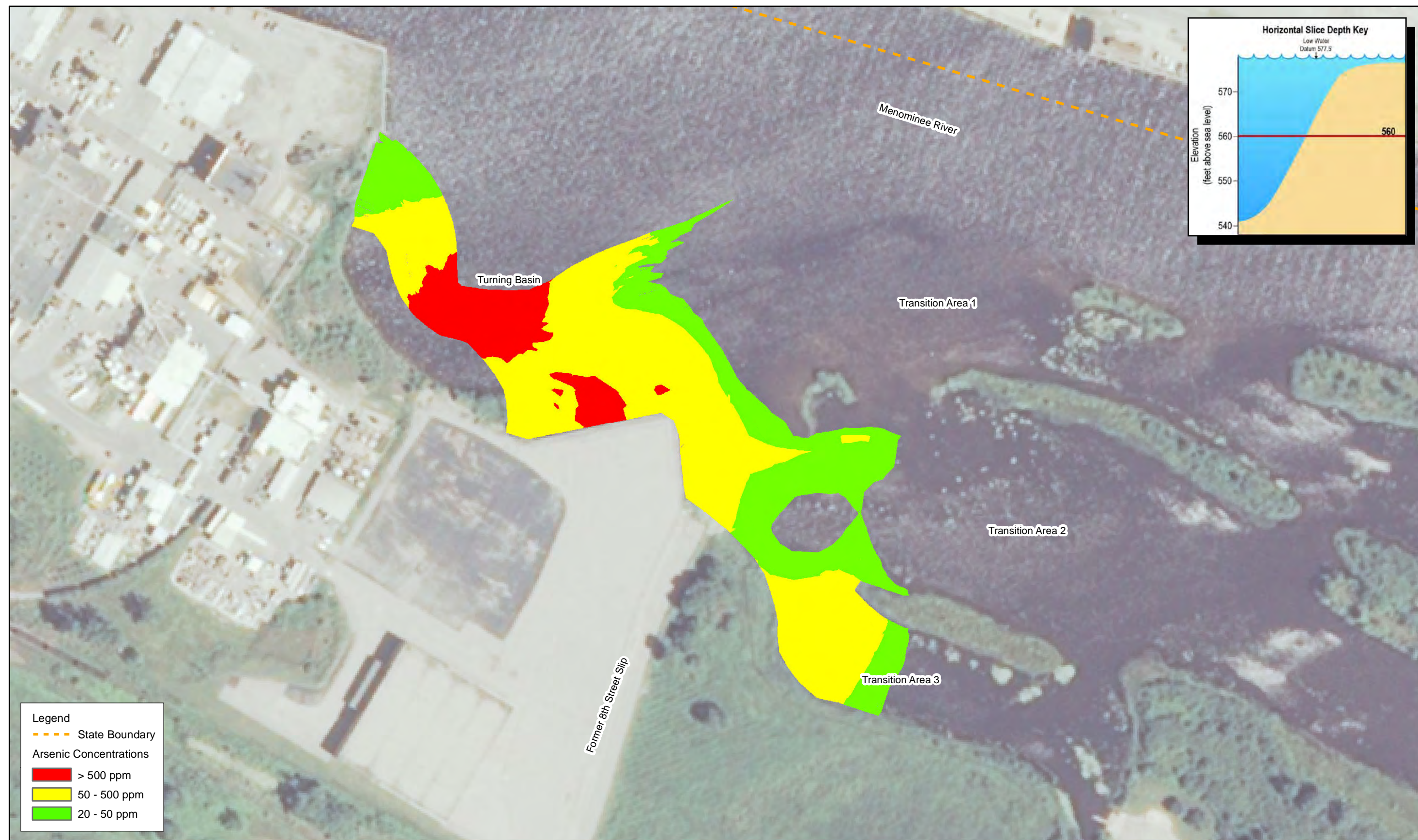
Figure 15H Horizontal Slice of Project Area, Arsenic Concentrations Elevation 560' Tyco Fire Products LP Facility Marinette, WI
