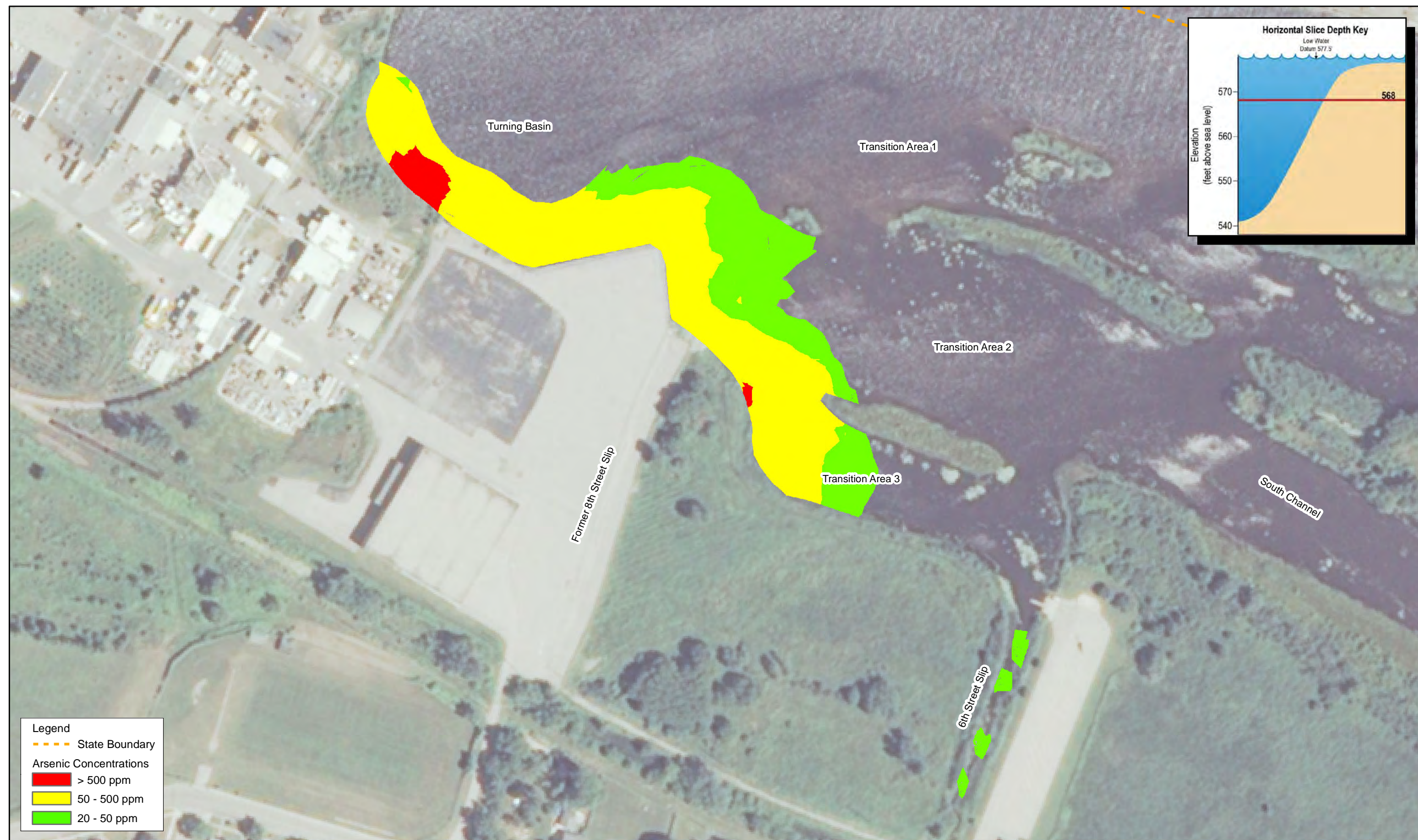
Figure 15L Horizontal Slice of Project Area, Arsenic Concentrations Elevation 568' Tyco Fire Products LP Facility Marinette, WI
