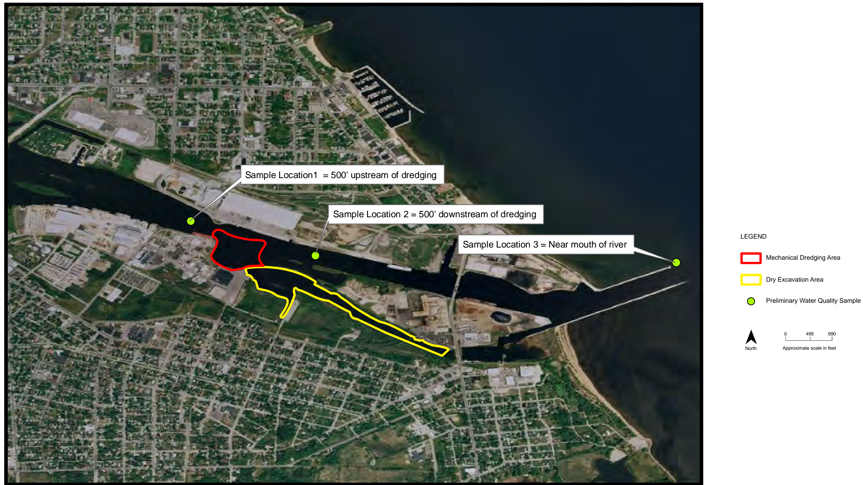
FIGURE 23 Preliminary Water Quality Sampling Locations During Dredging Tyco Fire Products LP Facility Marinette, WI
