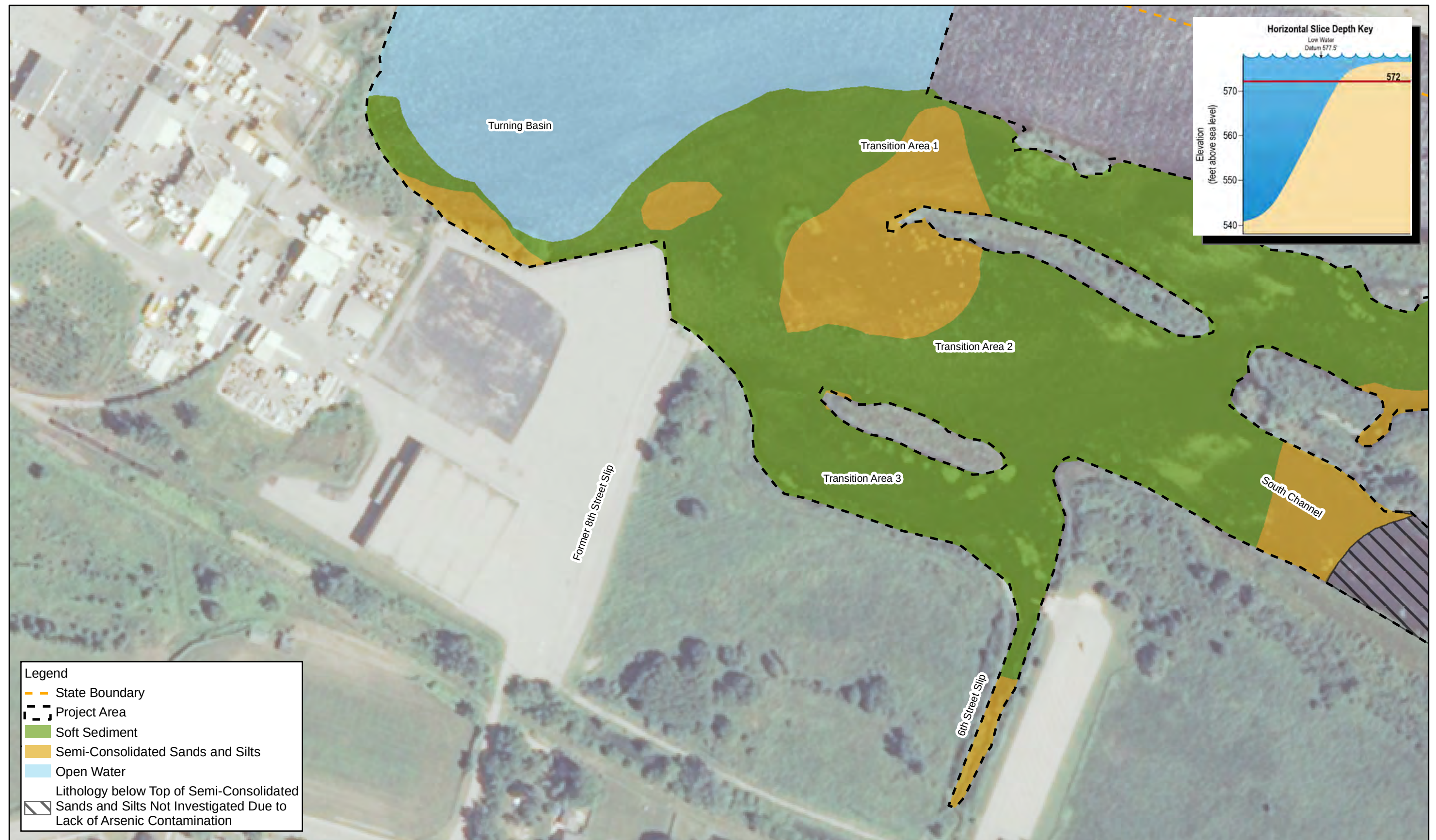
Figure 11N Horizontal Slice of Project Area Lithology Elevation 572' Tyco Fire Products LP Facility Marinette, WI
