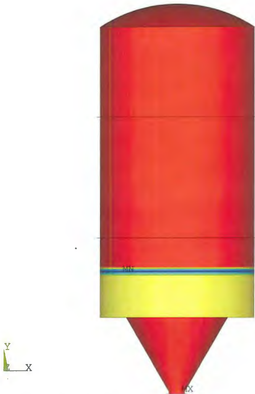
Figure 4-4 - Min Principal Stress for Operating Case - Weight + Hydrostatic Pressure (Full)
