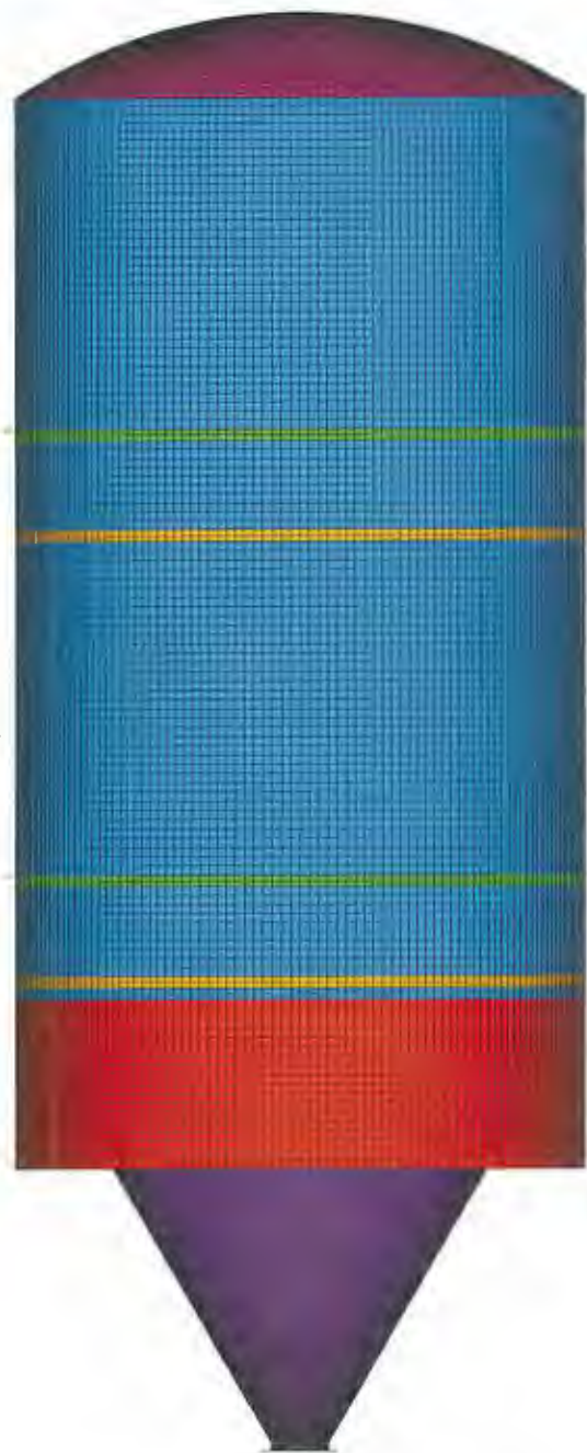
Figure 3-3 - ANSYS Finite Element Model of Storage Tank
