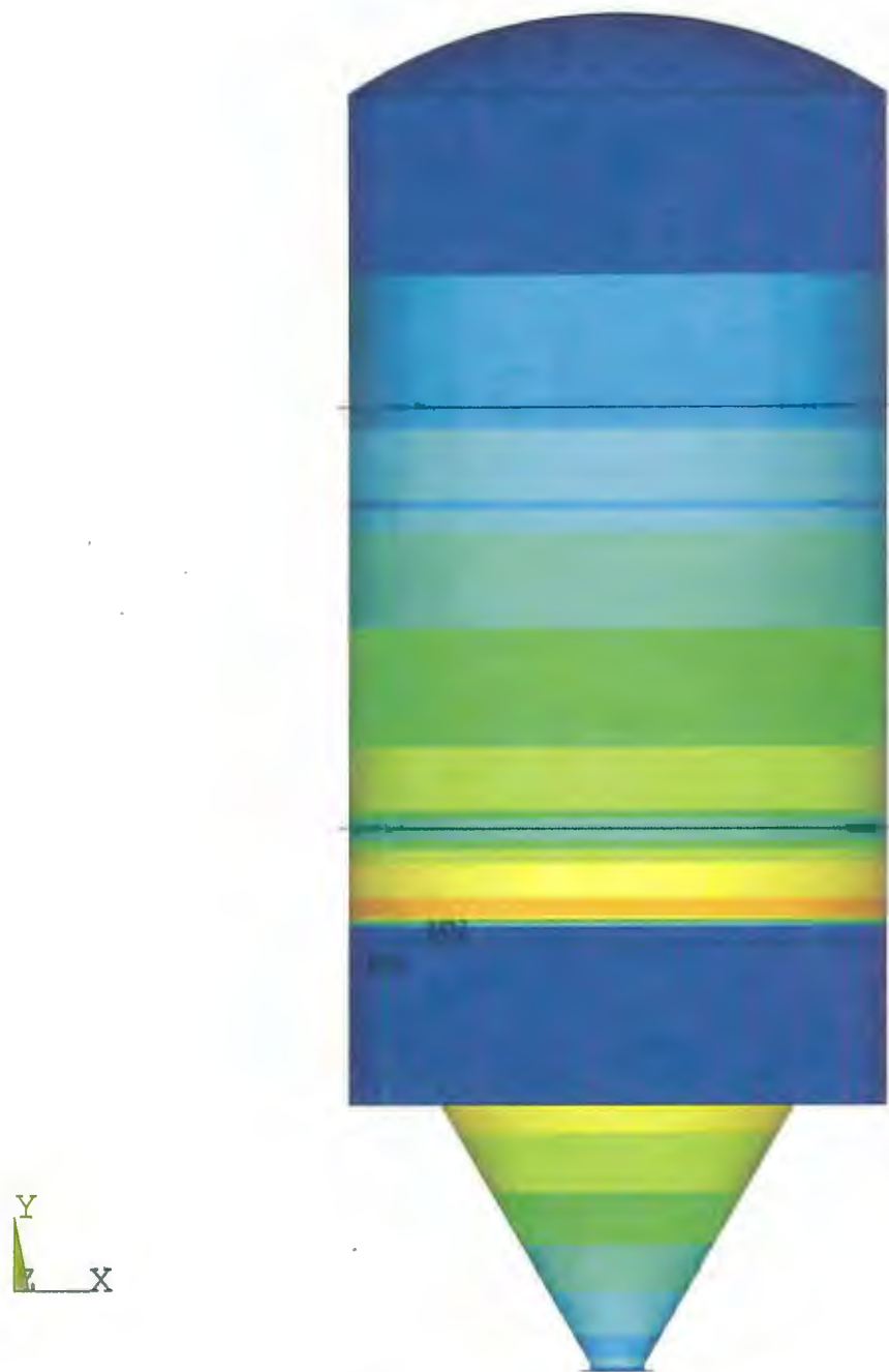
CBE 11 001 Shell Model (CBE Vessel): Max Principal stress
