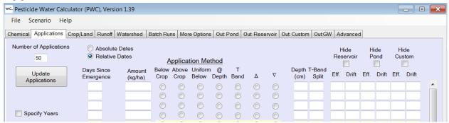
**Number of Applications:** Up to 50 applications (of the pesticide) per year can be specified. When the number of applications is altered, the user must click the *Update Applications* button and then only the relevant applications will be shown. The number of rows in the table will equal the number of applications (Note: The number of applications will also be registered at run time if the *Update Applications* button is not pressed).
