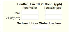
**Sediment Pore Water Fraction:** This is the fraction of pesticide in the benthic region that resides in the pore water.
