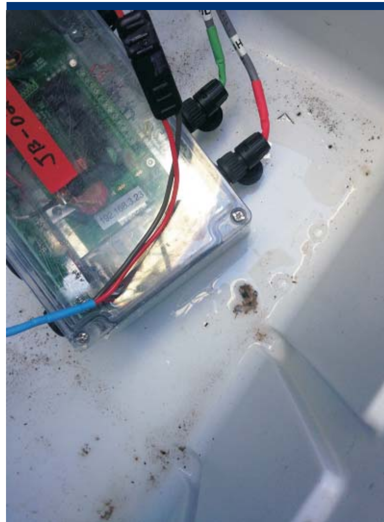
Photo 32 Viper station at JB02 is disassembled and water is visible in bottom of enclosure (not from leakage, but from condensation).
