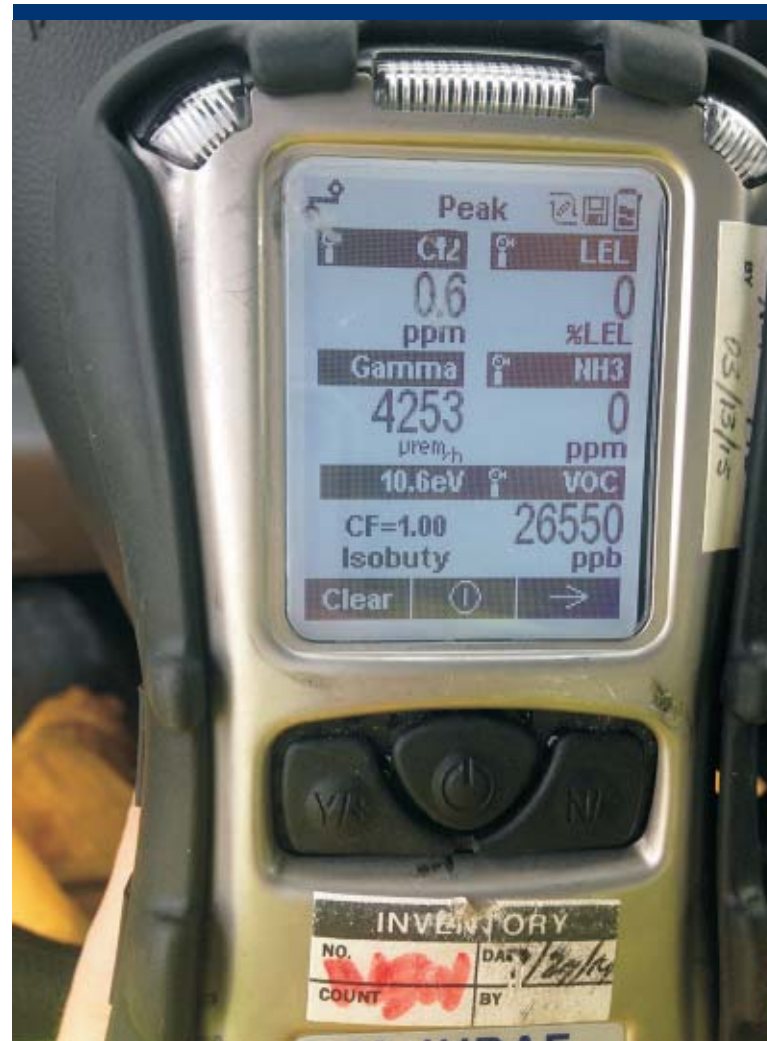
Photo 21 Peak gamma detection believed to be sensor error. Peak VOC due to bump test.
