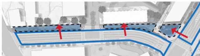
Figure 93 Diagram of the sub-watershed and treatment areas along Barton Springs Road. Areas outlined in blue represent the sub-watersheds within the site; shaded blue zones represent treatment areas; and red arrows indicate the flow direction from sub-watershed to treatment area.
