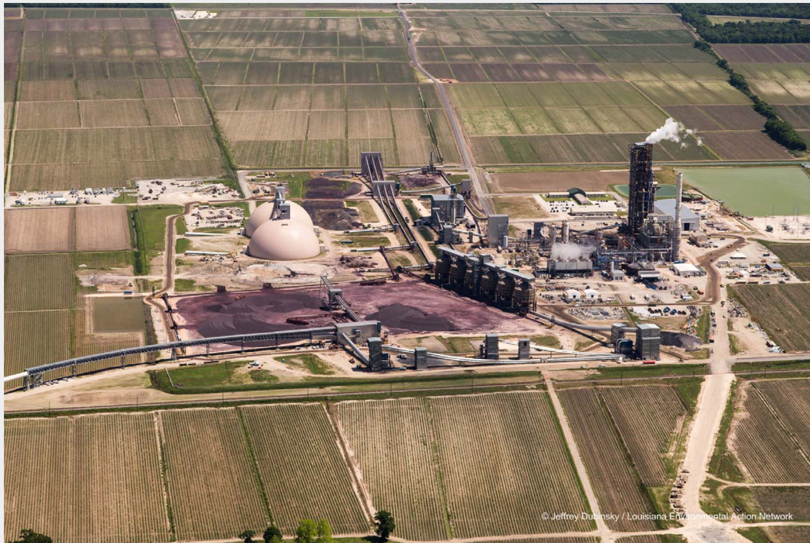
Nucor Steel (Convent, LA) Direct Reduction Iron (DRI) Plant Consumes 30 Million mmbtus/year of natural gas.
