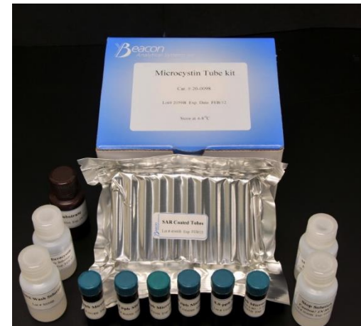
Beacon toxin tube kit (0.3 – 5.0 \mu\text{g/L} )
