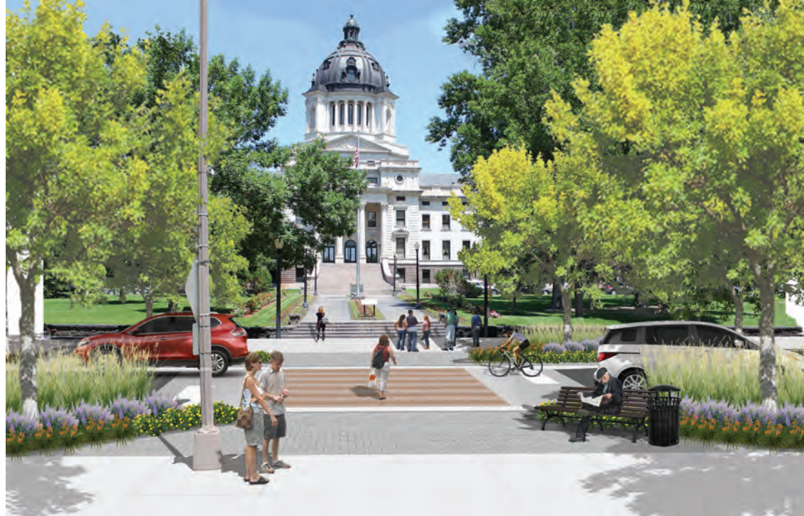
Figure 14: Design concept for the pedestrian crossing over East Capitol Avenue directly south of the capitol building. Stormwater planters and street trees could be added to a mid-block bulb-out. The added vegetation could help frame the capitol building and draw visitors' attention toward the historic building. A textured and colored pedestrian crossing would be more visible to drivers and would be safer for pedestrians crossing the street.
