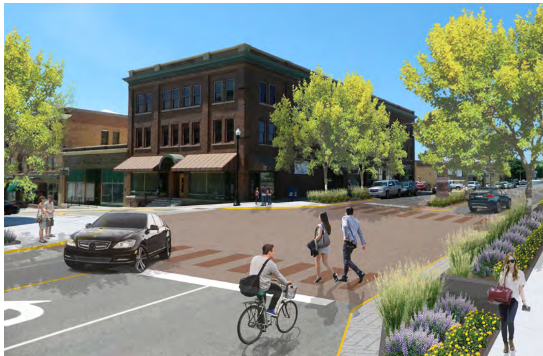
Figure 18: Design concept for the intersection of East Capitol Avenue and Upper Pierre Street. A colored and textured intersection makes pedestrian crossings more visible. Stormwater planters and street trees have been added along the rights-of-way and in a center median. These elements work together to calm traffic, making bicyclists and pedestrians crossing the street safer.
