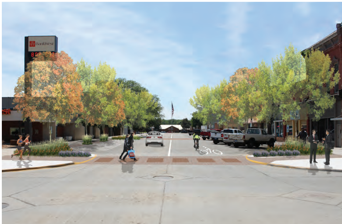
Figure 27: Design concept for the block-long segment of South Pierre Street between Dakota Avenue and Missouri Avenue. Framing the American Legion at the terminus of South Pierre Street, the stormwater planters and street trees add shade and visual appeal along South Pierre Street. Bike lanes and more visible pedestrian crosswalks can keep people safer as they cross the street.
