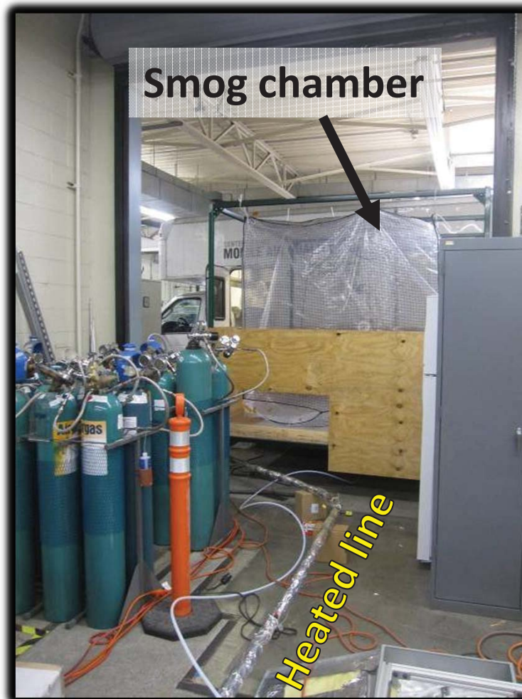
Secondary aerosol production investigated with portable smog
