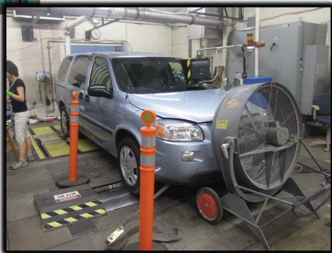
Light-duty vehicles tested using cold start Unified Cycle
