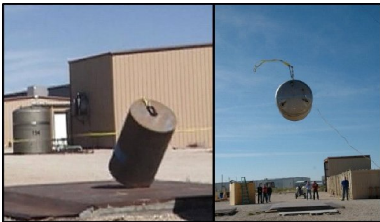
Figure 4. Drop testing the Shielded Container (left pane) and inside a shipping container (right pane).
