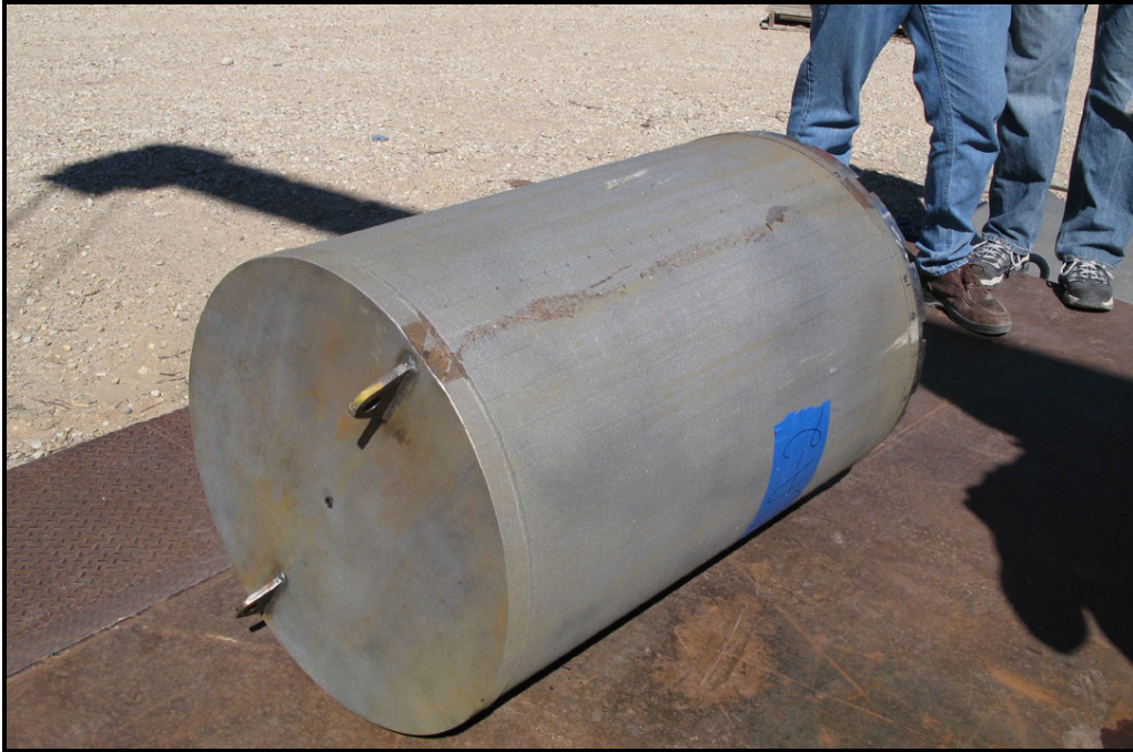
Figure 4-10 – SCA-2 Body Damage Overall, Side Drop Test
