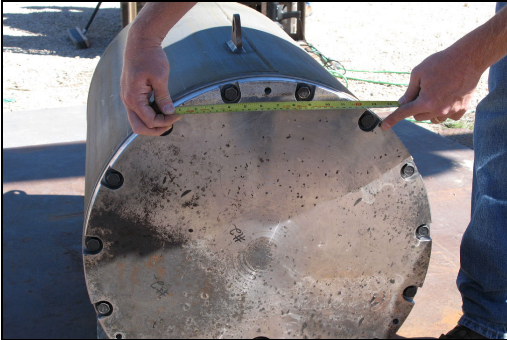
Figure 4-8 – SCA-2 Lid Damage Front View, Top-Down, Near-Vertical End Drop Test
