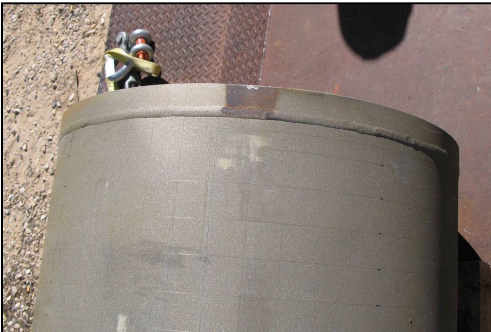
Figure 4-5 – SCA-1 Body Damage, Top-Down, Center of Gravity-Over-Corner Drop Test
