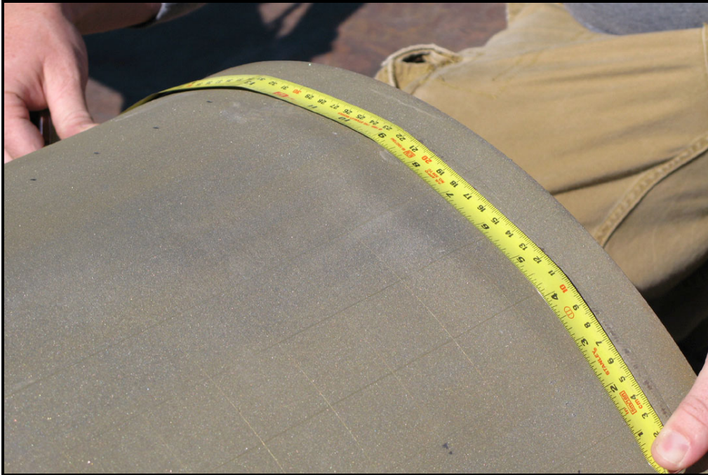
Figure 4-6 – SCA-1 Body Damage Top View, Bottom-Down End Drop Test
