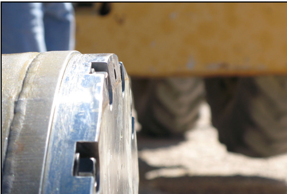
Figure 4-9 – SCA-2 Lid Damage Side View, Top-Down, Near-Vertical End Drop Test
