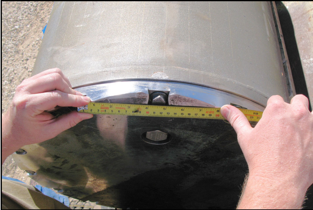
Figure 4-4 – SCA-1 Lid Damage, Top-Down, Center of Gravity-Over-Corner Drop Test
