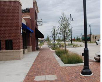
Figure 12 | These photos from Kansas City, MO (top) and Greensburg, KS (bottom) show how green infrastructure solutions can be incorporated into the amenity zone of the street right-of-way.
