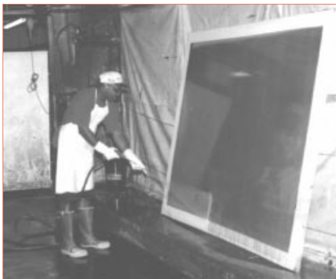
Screen reclamation with a high-pressure water system
