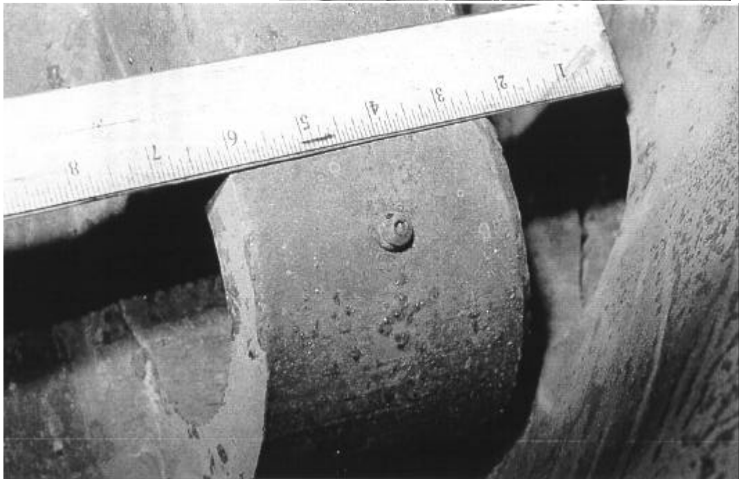
Figure E-12: Photograph shows the head of the machine screw protruding from the portion of the fractured pin. The pin is shown extended slightly out from the surface of the flange, or disk "ear", from which the valve shaft was ejected.
