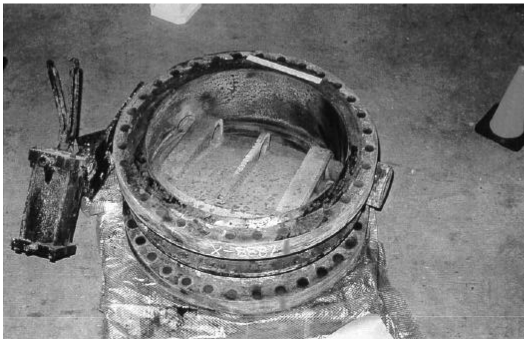
Figures E-9 and E-10: Photographs of two views of the disassembled subject 36" Clow check valve. The pneumatic actuator assembly can be seen in both views. In the lower photograph, the hole directly below the 12-inch ruler formerly contained the valve's drive shaft. This is where the shaft blow-out and flammable gas release occurred.
