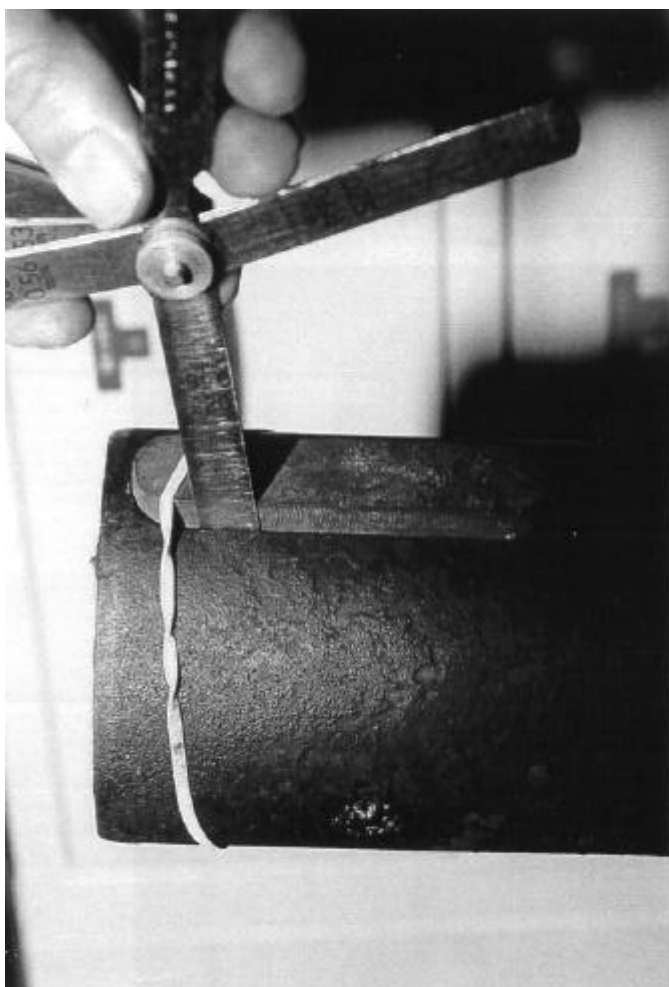
Figure E-13: Photograph shows the metal key intended to help mechanically connect the drive shaft to the valve disk.
