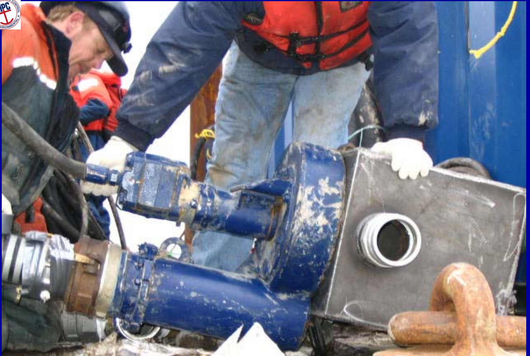
A hydraulic submersible pump mounted on a steel debris box. The debris box decreases the likelihood that rock or other object will jam the pump.
