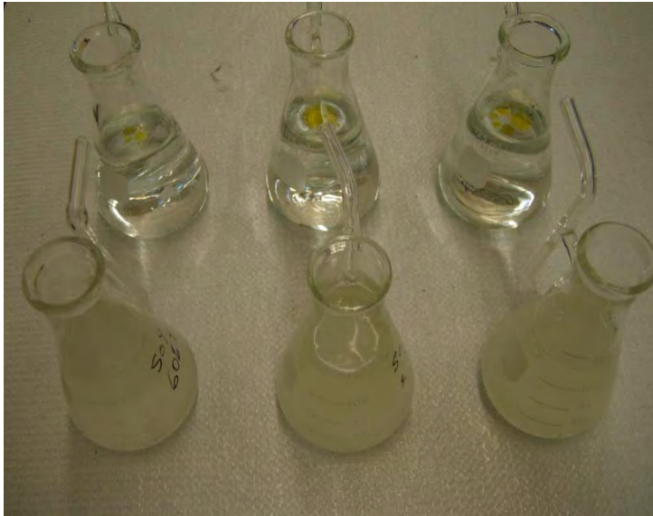
Low Energy Mixing Swirling Flask Test
