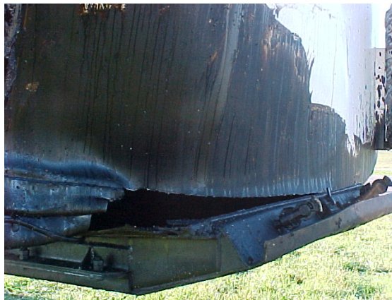
Fig 2 – Tank rupture detail.
