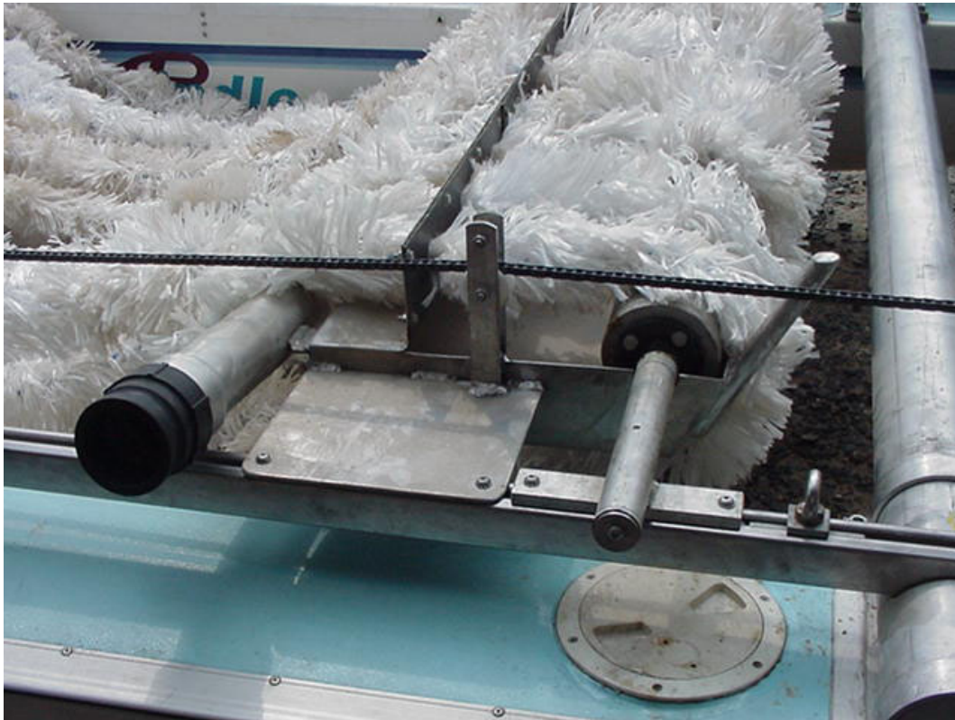
Figure 60. Rope mops passing through the stripper, camlock connection, and collection tray.
