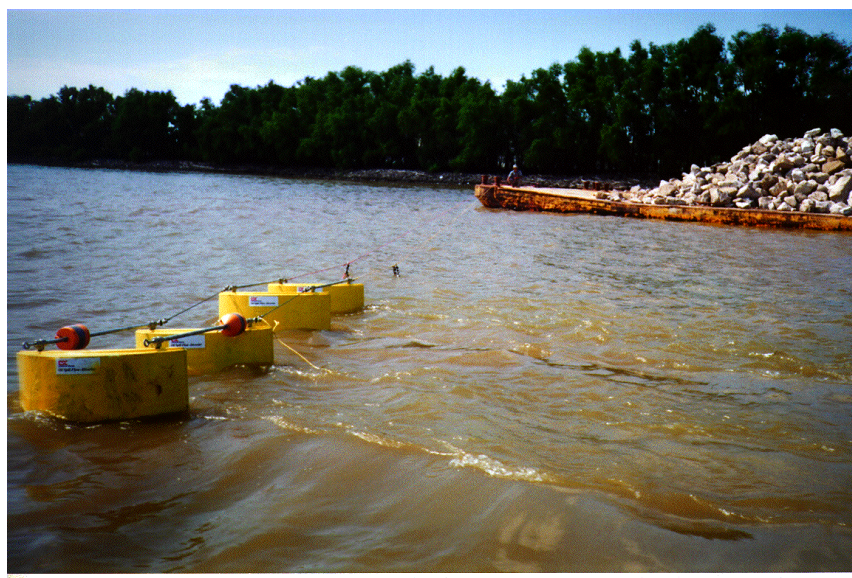
Figure 6. Two Catamarans Deployed from a Stationary Barge, Mississippi River 1.5 knots
