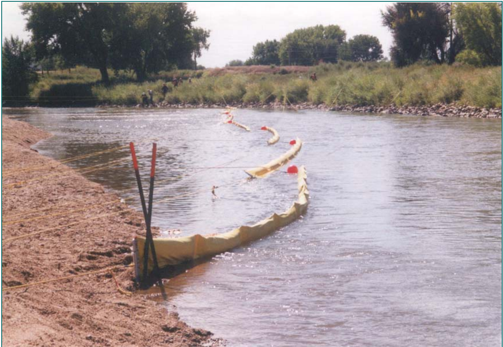
Bank to Bank Rope Anchor System South Platte River – Colorado
