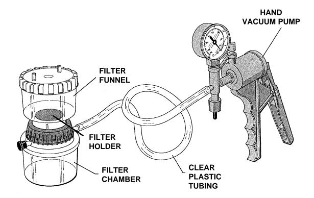
Figure 8-4. Filtration apparatus for preparing chlorophyll and biomass subsamples for periphyton. Modified from Chaloud et al. (1989).
