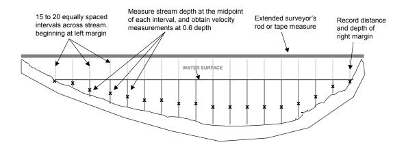
Figure 6-1. Layout of channel cross-section for obtaining discharge data by the velocity-area procedure.
