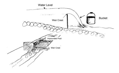
Figure 6-3. Use of a portable weir in conjunction with a calibrated bucket to obtain an estimate of stream discharge.
