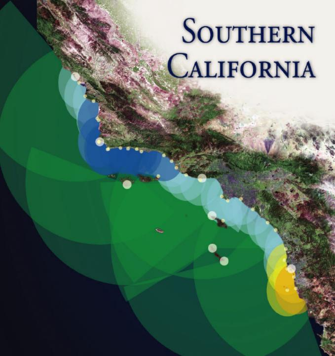
SITE LOCATIONS FOR HIGH RESOLUTION OCEAN CURRENT MAPPING HF RADAR WITH ~40KM RANGE
