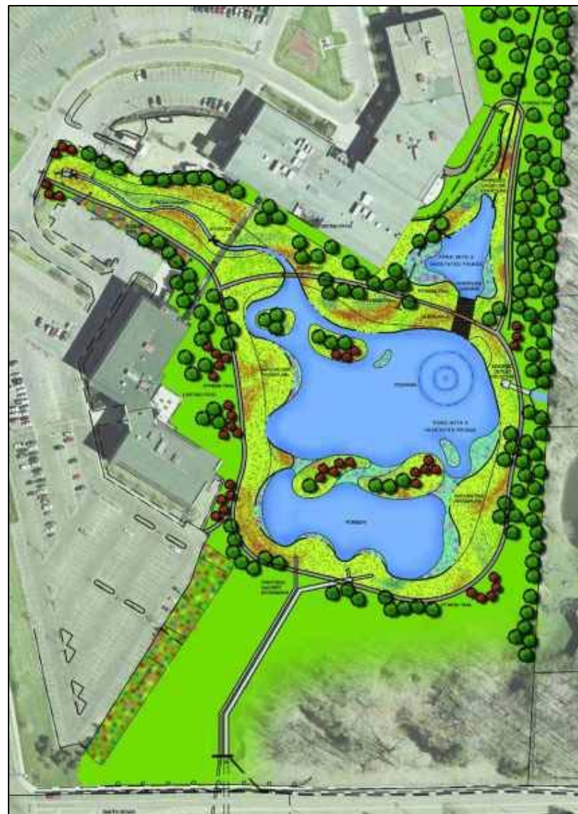
The vegetated areas surrounding this urban stream, pond and wetland restoration area serve as urban filter strips to help treat runoff. This example is located in Akron, Ohio.
