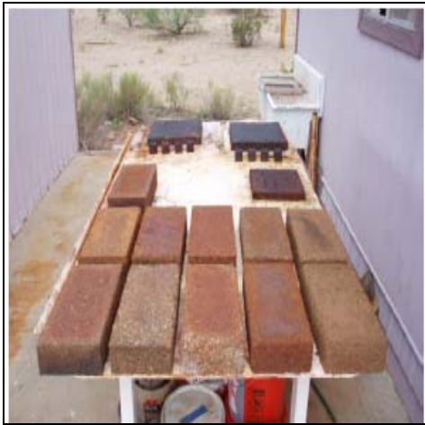
Bricks made from adobe and glass
