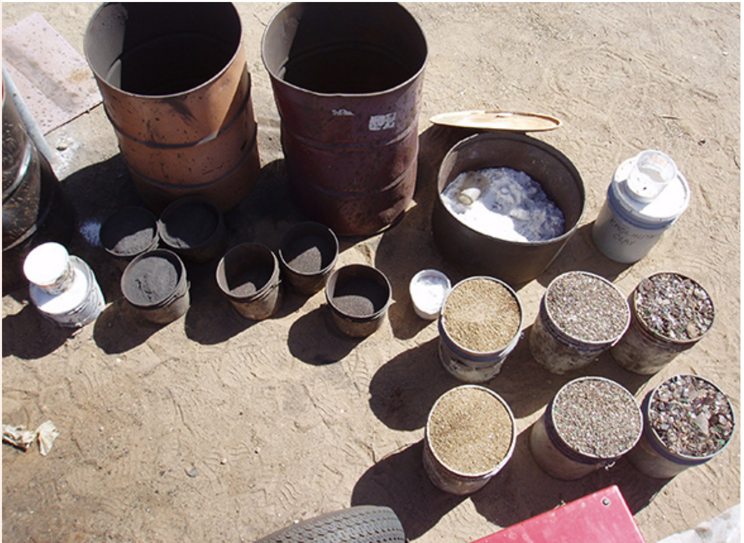
Materials combined to create building material including pulverized glass and steel dust waste. Photo courtesy of TOCC.
