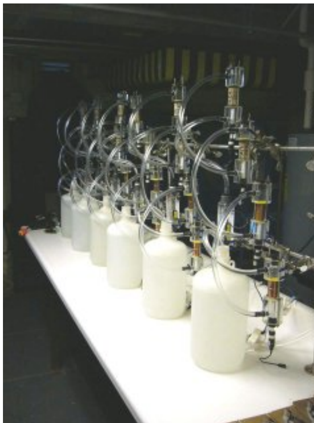
Exhibit 2.3.1 Photograph of Electrochemical Polarization Cell Used in the EC Pipe Loop System
