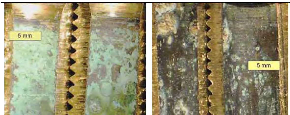
Figure F.128 Brass Supply Tubes for Faucet 08_FB02 (Site F.1). The cold water supply (left) and hot water supply (right)
