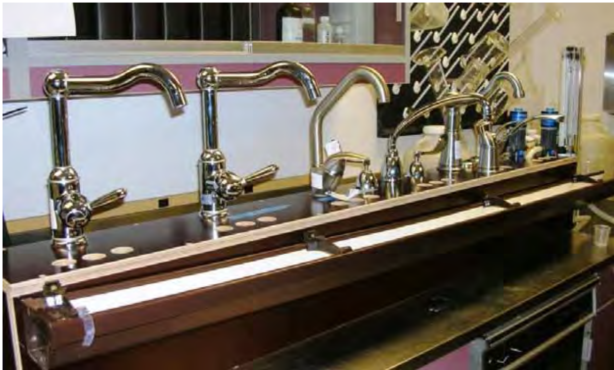
Figure C.2 Portland Water Bureau faucet test rig.
