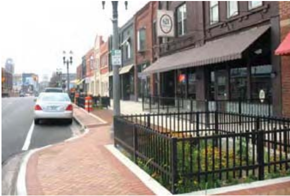
Michigan Avenue rain gardens in planter boxes in Lansing, MI. Source: Tetra Tech
