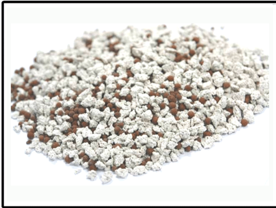
FIGURE 12: Example of light-weight growing medium (expanded clay aggregate or vermiculite and other light-weight, high water storage capacity components). 18
