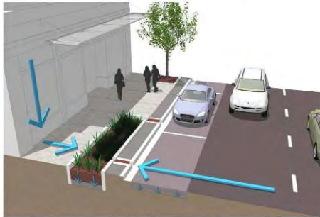
Planters and Pervious Paving
