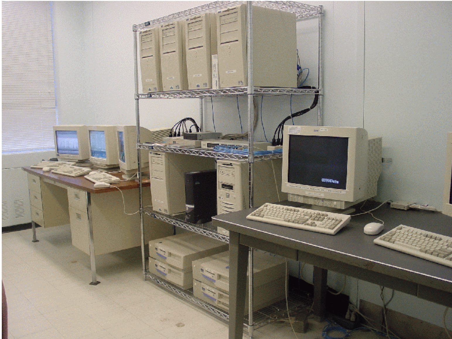
Figure 5-5. MiniMUSE Parallel Computing Cluster at ORD/NERL/ERD.
