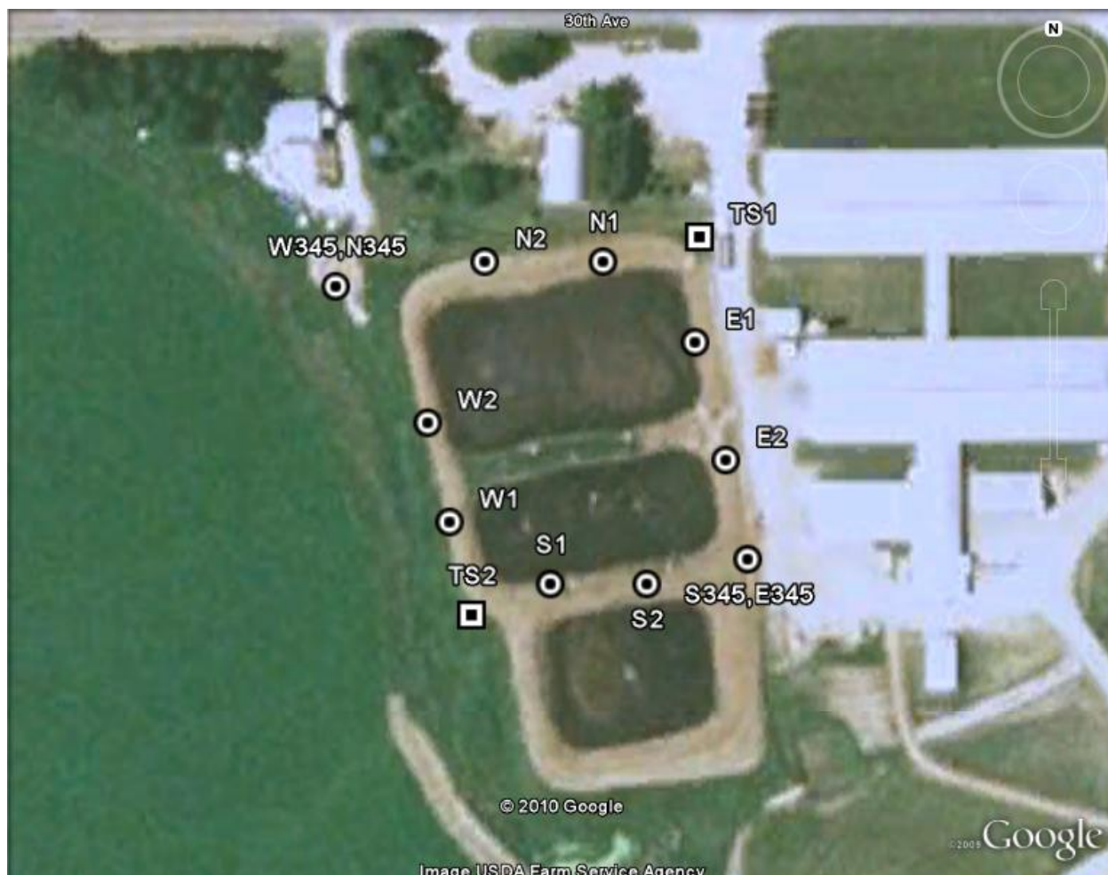
Figure 1-2: Locations of instrumentation around the lagoon under measurement. Retro-reflectors are indicated according to side (N,S,E,W) with 345 indicating the location of a tower. TDLAS/scanner locations are indicated by TS. The location of the two S-OPS are indicated by the solid yellow lines. The instrumentation trailer was located in the northeast corner of the lagoon.
