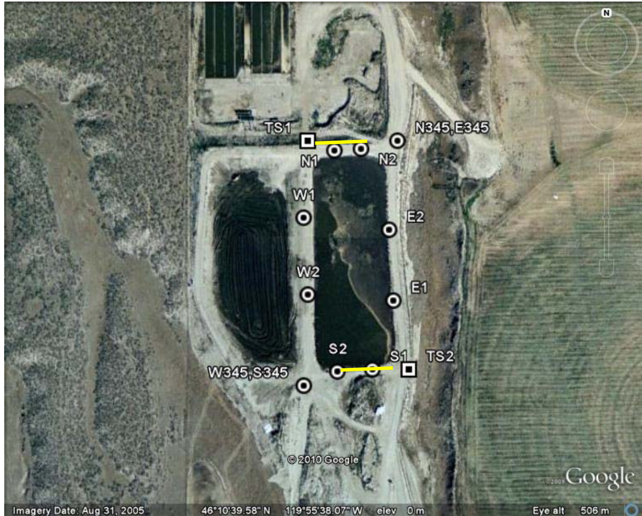
Figure 1-2: Locations of instrumentation around the basin under measurement. Retro-reflectors are indicated according to side (north, south, east, and west) with 345 indicating the location of a tower. TDLAS/scanner locations are indicated by TS. The locations of the two S-OPS are indicated by the solid yellow lines. The instrumentation trailer was located in the northeast corner of the basin.
