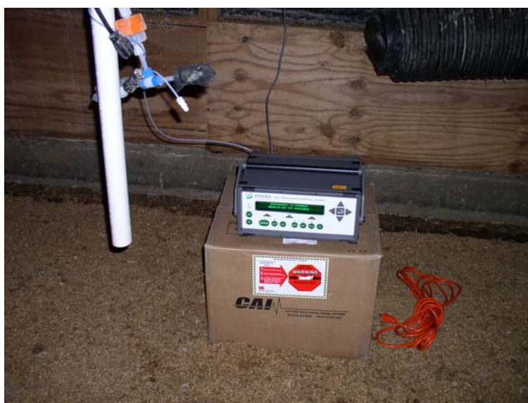
Figure 14. One of the three in-house INNOVA analyzers used to compare readings to its counterpart inside the MAEMU.
