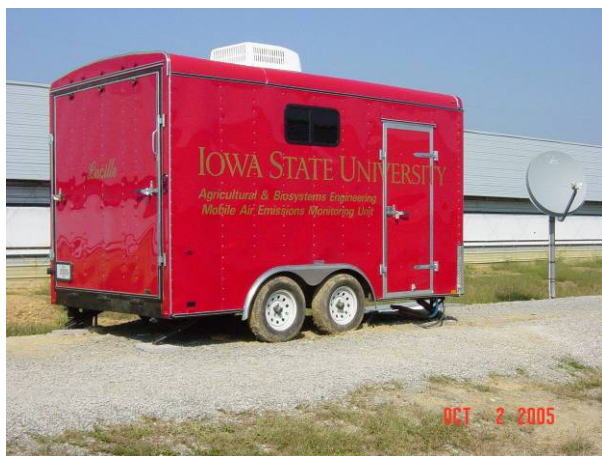
Figure 4. Environmentally-controlled Mobile Air Emissions Monitoring Units (MAEMU).
