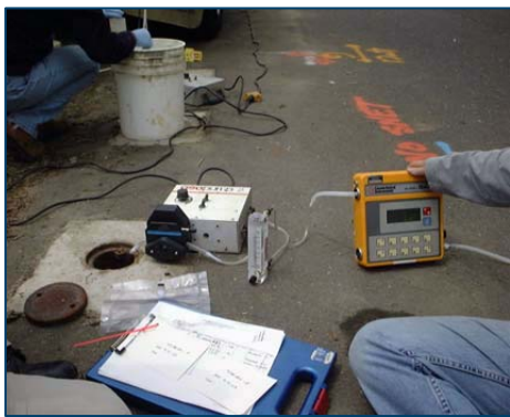
Figure 1: Sampling train (peristaltic pump, flowmeter, landfill gas meter) for collection of samples from dedicated vapor probes
