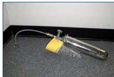
Figure 4: Sub-slab sampling with 1-L Canister
