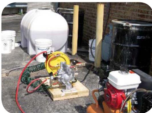
*ISCO system installed behind a small drycleaning facility.*
