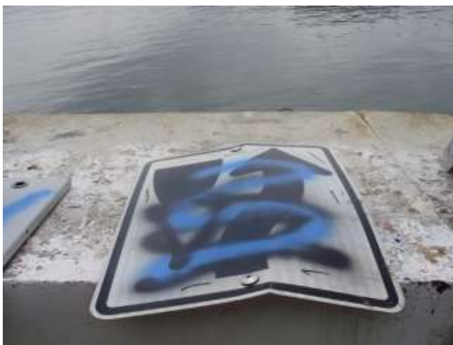
Figure 5-15. Coval coating on no parking sign with graffiti
