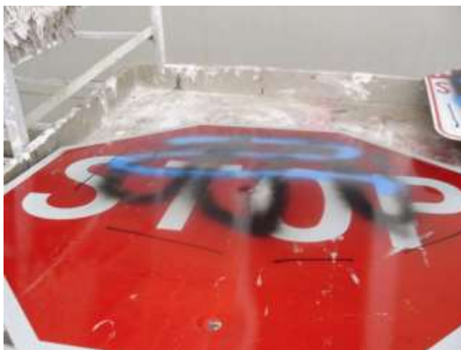
Figure 5-16. Coval coating on stop sign with graffiti
