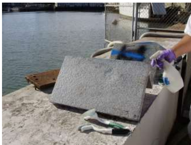
Figure 5-11. Graffiti resistant coatings on granite after graffiti removal
