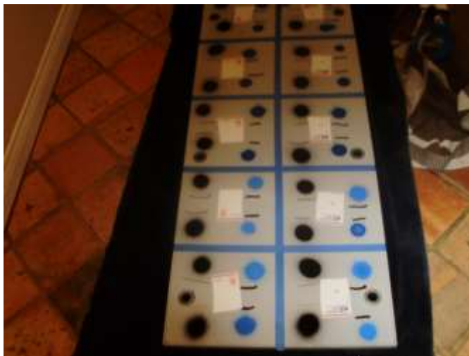
Figure 4-8. Masked off sections on fiberglass panel
