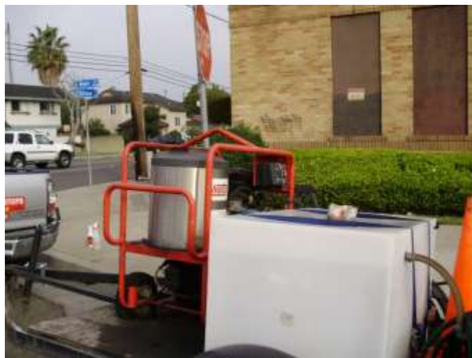
Figure 2-5. Soda blasting system
