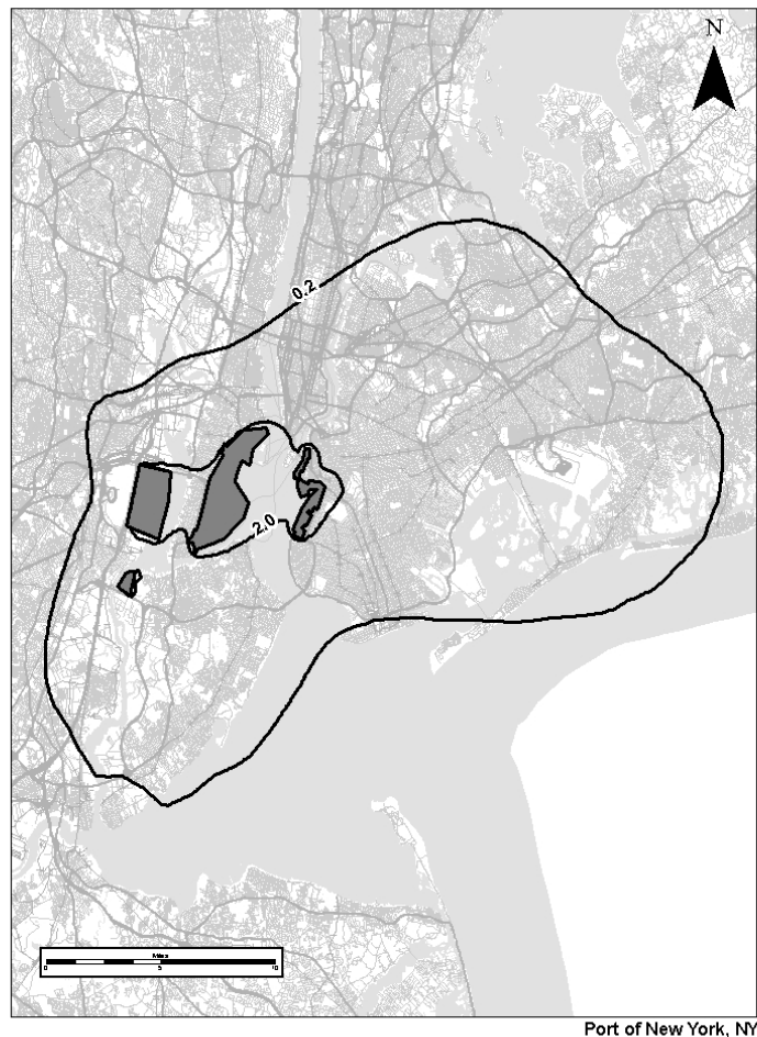
Figure 2-5 Concentration Isopleths of New York, NY Harbor Area Resulting from All Emission Sources.
