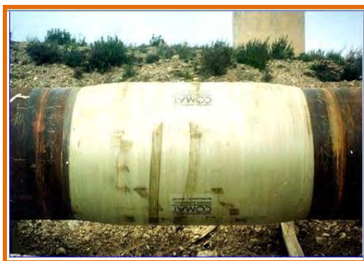
Figure 5: Composite crack arrestor for gas pipelines before and after a fracture propagation test.
