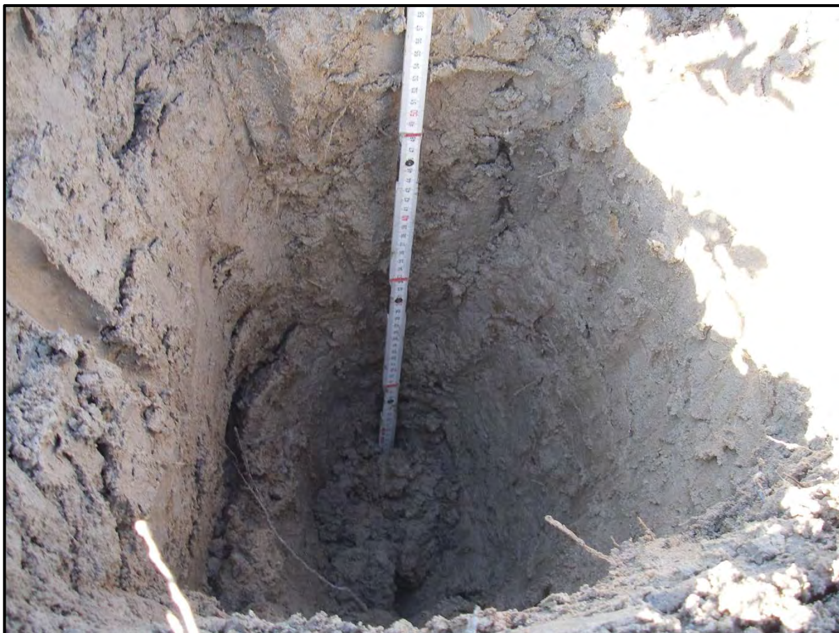
Figure 13. Shovel test to a depth of 84 cm where ground water was encountered. September 18, 2013.
