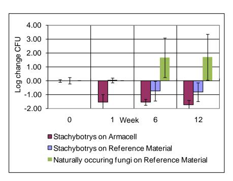
Figure 3-2. Log change in *Stachybotrys chartarum* inoculated on the test material over 12 weeks on the insulation reference material and Armacell.
