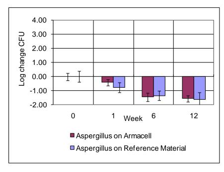
Figure 3-1. Log change in *Aspergillus versicolor* inoculated on the test material over 12 weeks on the insulation reference material and Armacell.
