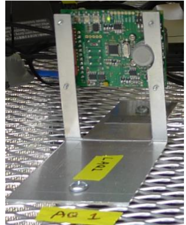
Figure A-8. Aeroqual board inside the chamber (Figure A-1) during field deployment.
