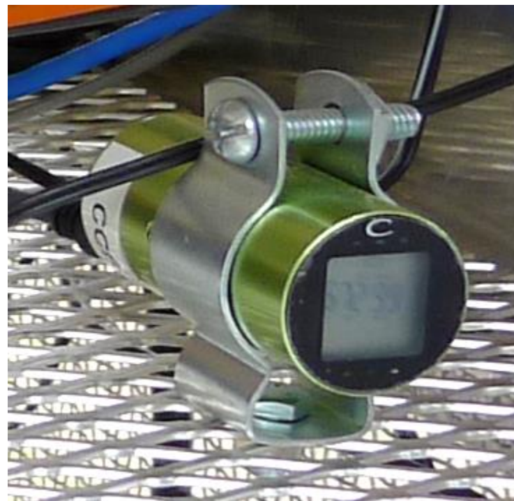
Figure A-10. CairClip sensor inside the chamber (Figure A-1) during field deployment.
