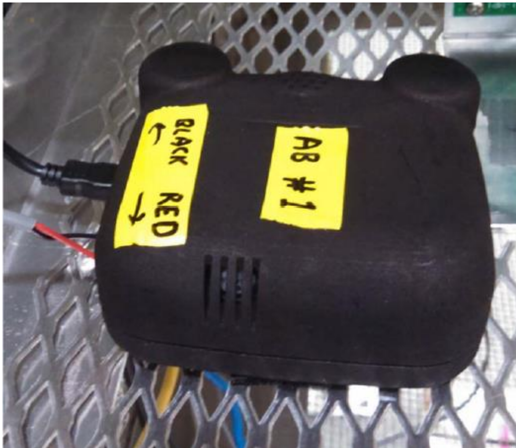
Figure A-4. Airbeam air monitoring device inside the chamber (Figure A-1) during field deployment.
