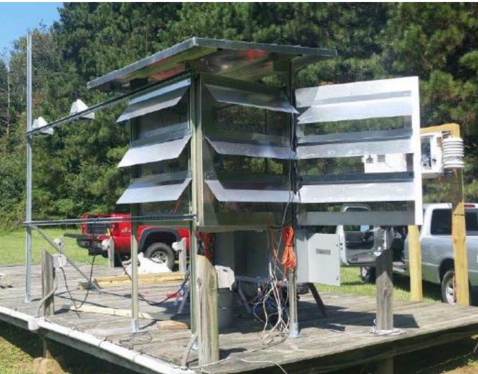
Figure A-1. Housing for the CAIRSENSE ad-hoc sensor testing in Atlanta.
