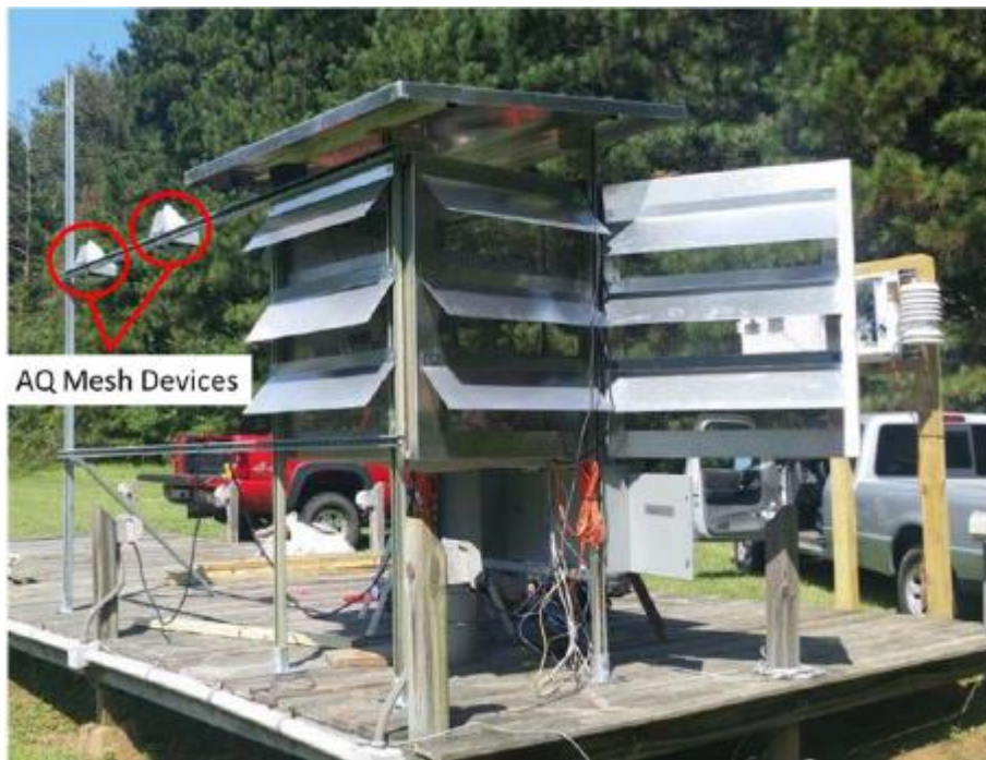
Figure A-11. AQ Mesh field setup.
