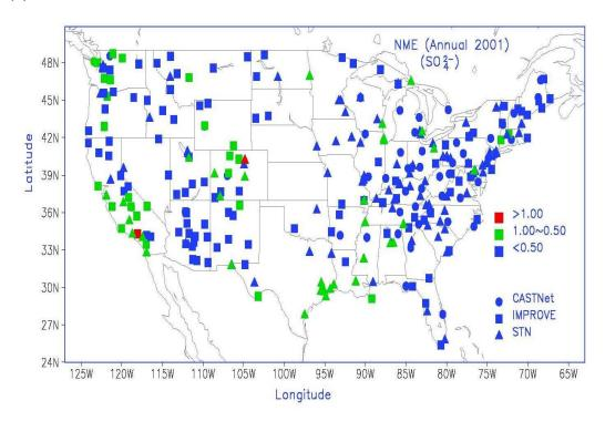
**Figure 1.** (c) East and west monthly mean sulfate (SO<sub>4</sub>) 2001 IMPROVE, CASTNet, and STN observations versus CMAQ predictions; (d) Annual mean SO<sub>4</sub> performance at IMPROVE, CASTNet, and STN sites.
